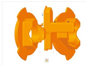
Put the cam disks in the lower shafts, keep in mind that they have to fit in the lower pressing units.
