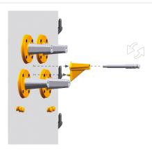
Remove the rod of the blade support and the rear blade holder. Clean properly the area.
